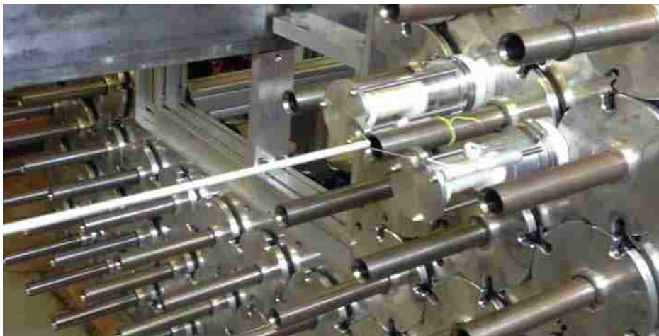
Figure 2.3: Test Specimen Being Manufactured on Prototype IsoTruss Machine
